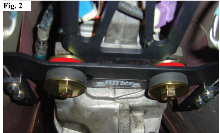
Example Install of TR-3650 with Stiffeners Loop
