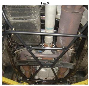
Complete Install w/Driveshaft Safety Loop option
